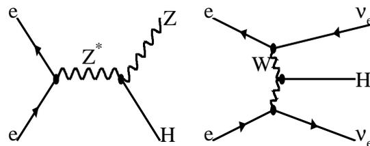
Figure 1. Higgs production through Higgsstrahlung (left) or boson fusion (right).
